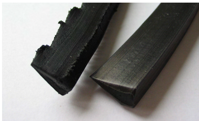
Figure 9: Test result from a Garvey test with two rubber compounds.
